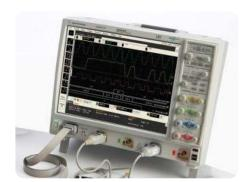
Integrated mixed-signal oscilloscope lets you trigger across time-correlated analog and digital channel combinations.
